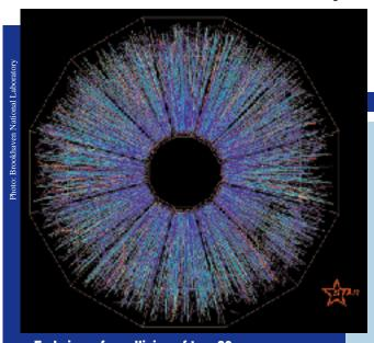
End view of a collision of two 30billion-electron-volt gold beams in the STAR detector at the Relativistic Heavy Ion Collider at Brookhaven National Laboratory. The beams travel in opposite directions at nearly the speed of light before colliding.
