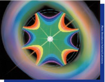
A representation of the magnetic field created by one of the 1,740 superconducting magnets in the Relativistic Heavy Ion Collider. RHIC collides speeding heavy ions and polarized protons in an effort to recreate a state of matter not seen since moments after the Big Bang.
