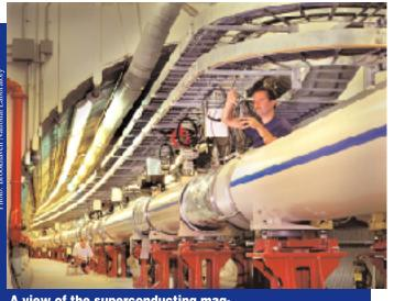
A view of the superconducting magnets at Brookhaven's Relativistic Heavy Ion Collider. As gold particles zip along the collider's 2.4 mile long tunnel at nearly the speed of light, 1,740 of these magnets guide and focus the particle beams.
