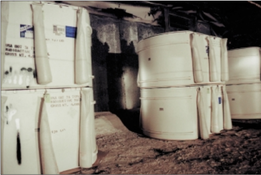
The six SWBs, comprising the initial TRU waste shipment to WIPP, in Room 7 of underground disposal Panel I
