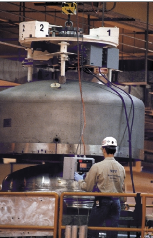
A TRUPACT-II container with its lid removed to facilitate inspection of the standard waste boxes (SWBs) inside
