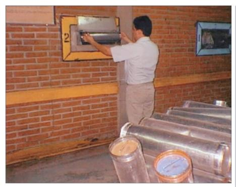
A worker at the Tuxtla Guttierez plant loading cylinders filled with pupae into irradiators
