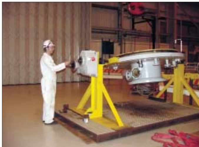
The turning rig for the ESW (essential service water) strainer lid developed by staff at Sizewell B (BE)
