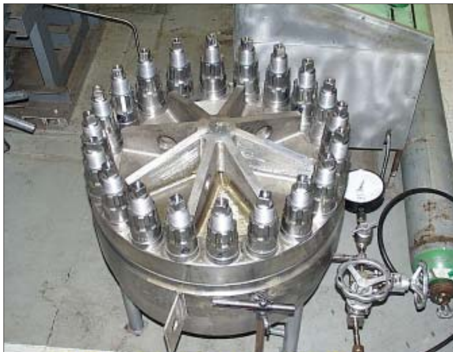
Testing of the new stainless steel gasket ring that seals the steam generator header covers at Dukovany (CEZ)
