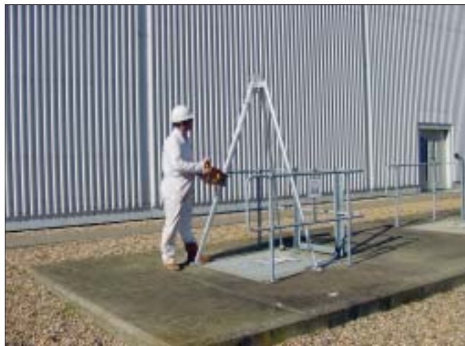
A tripod lifting frame for removal of sump pumps from cable tunnels (BE)
