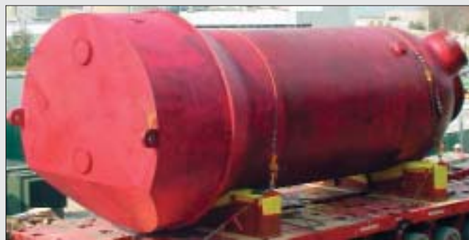
Calvert Cliffs-2's original steam generator lower assembly moves to a secure onsite location for storage.
