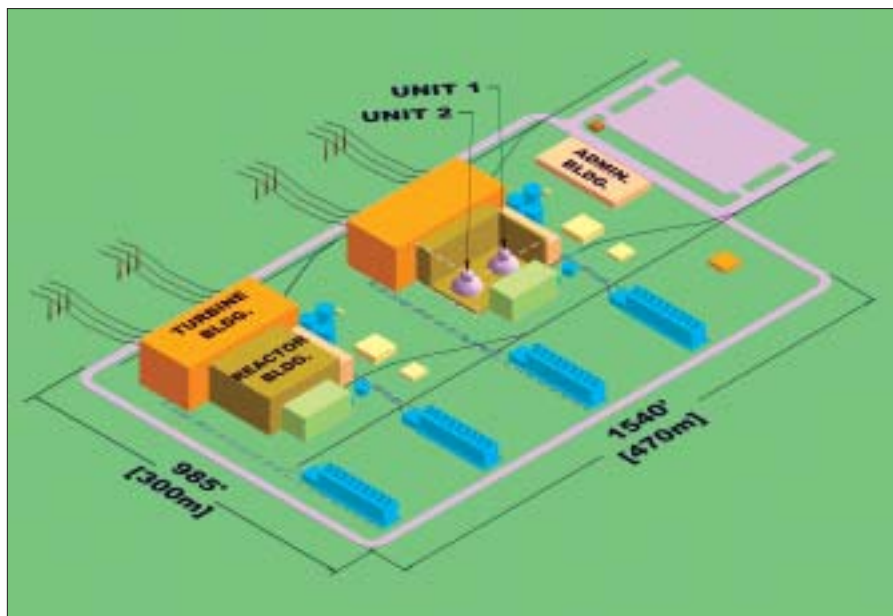
Fig. 10. IRIS two twin-unit plant layout arrangement
