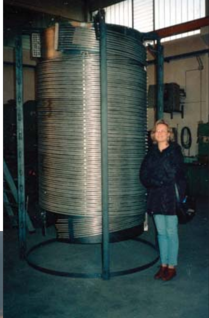
Fig. 4. Mock-up of IRIS helical coil steam generator
