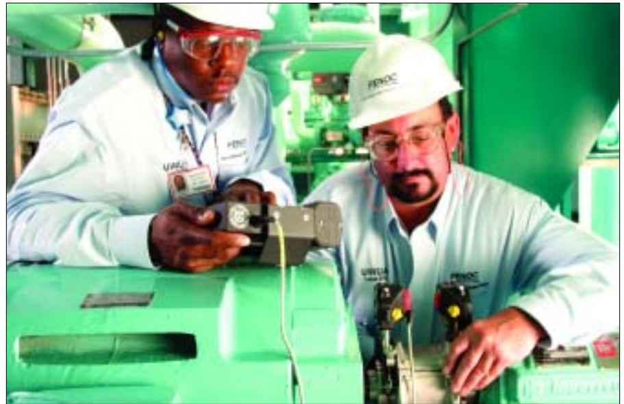
Perry maintenance mechanics Fred Barthany and Mark Paolillo practice pump shaft alignment during a training session on flow loops. (Photos: Tommy Thompson)
