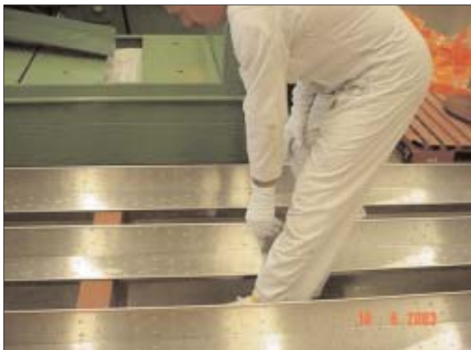
CRB being inspected for scratches and dents
