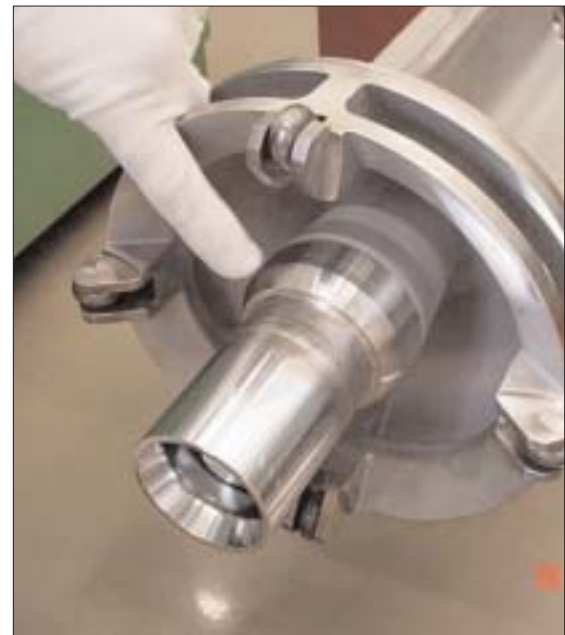
Velocity limiter, showing four new pin/rollers
