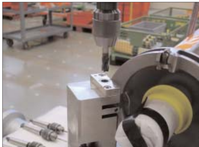
Drill above alignment fixture over velocity limiter roller
