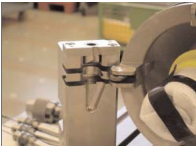
Drill alignment fixture for velocity limiter roller
