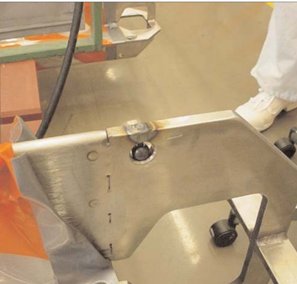
Drilled handle weld following pin/roller replacement
