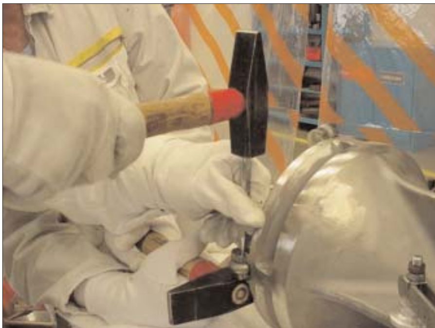
Pin being removed from CRB
