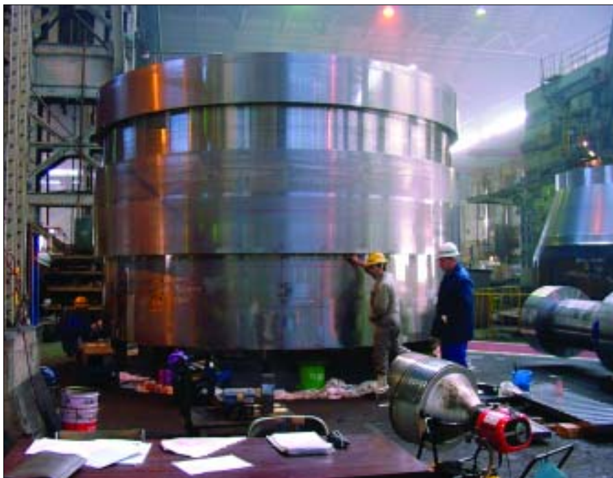
Fig. 4. The nozzle shell flange of the EPR's reactor pressure vessel
