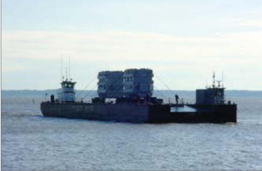
Two new generator step-up transformers are barged from Hampton Roads, Va., to the Surry nuclear power station in Gravel Neck, Va. (Photos: Dominion)
