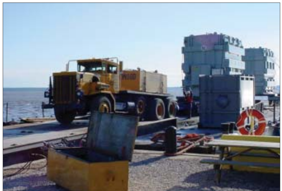
The transformers are then unloaded from the barge on the James River near Surry's intake canal.
