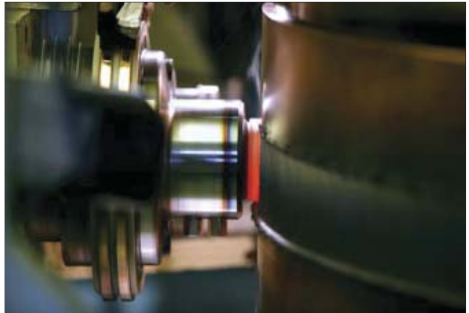
A shot of friction stir welding of a spent-fuel canister's copper lid, during testing at SKB's canister laboratory in Sweden. (Photo: SKB)
