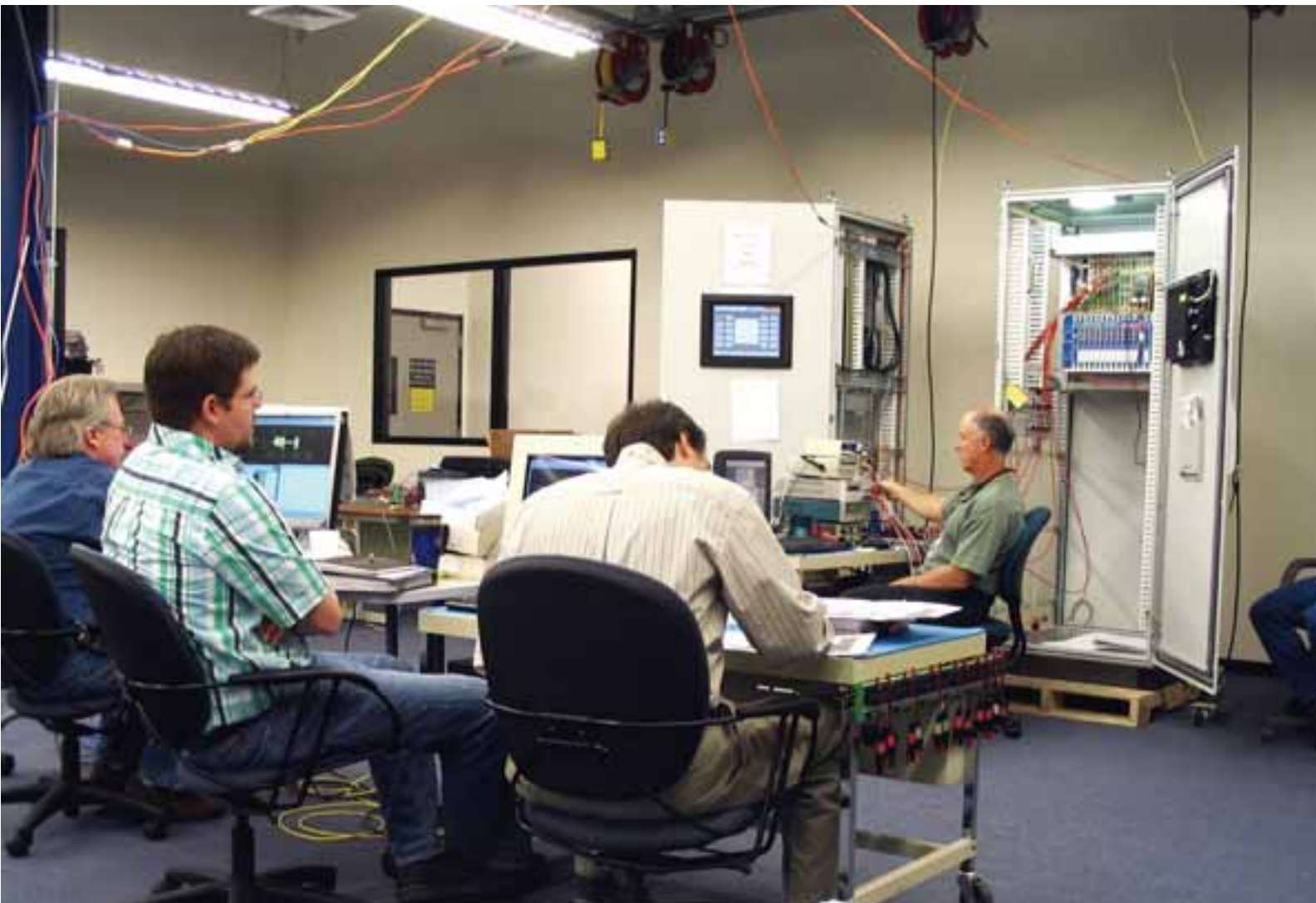
I&C technicians and engineers perform factory acceptance testing of Diablo Canyon's main feedpump vibration monitoring system.
