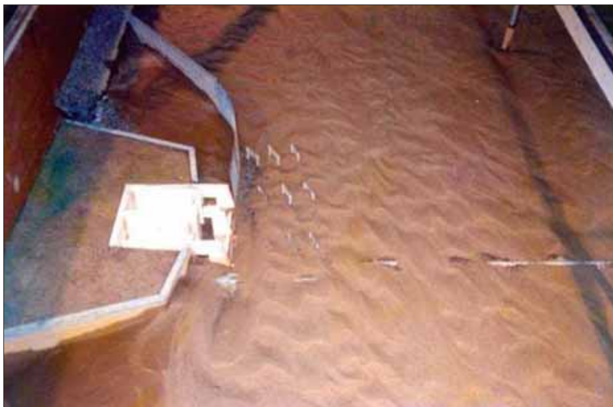
The University of Iowa's hydraulics laboratory model of the Cedar River and the Duane Arnold plant's intake structure (Photo: FPL Energy)
