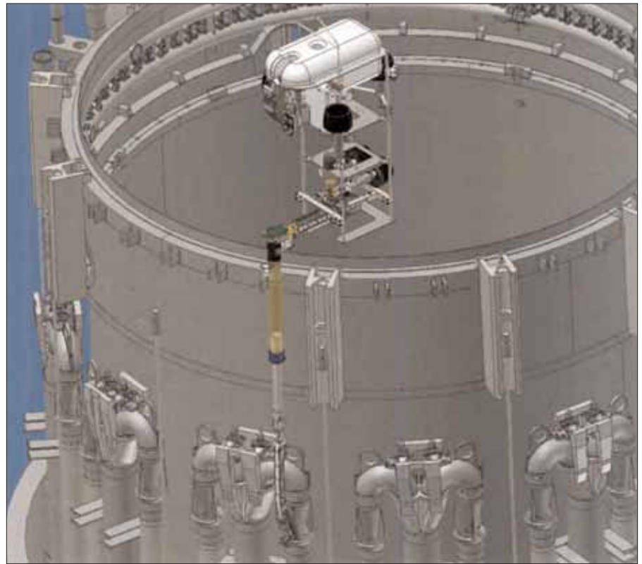
An illustration of Entergy Nuclear's Jet Pump Inspection Tool inside a reactor cavity (Graphic: Entergy Nuclear)
