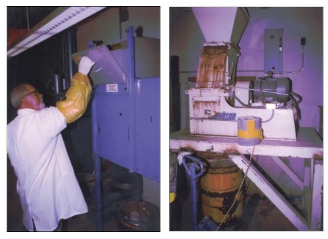
(Left) Loading scintillation vials into the vial crusher's bin. Liquid is drained into the bottle at the lower right, and the crushed glass and plastic go into a separate drum. (Right) The old vial crusher could only be used by climbing a ladder to dump vials into the funnel. This unit is now in the process of being decontaminated and removed for disposal.
