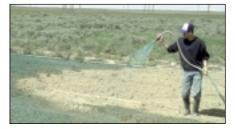
Applying kochia seeds to contaminated soil around Argonne National Laboratory– West in a test of phytoremediation. For a report on the results of the program so far, see article and photo essay beginning on page 49.
