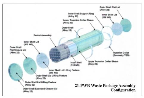
Fig. 8. Also a cylinder-in-a-cylinder, the SR design for the waste package uses an outer shell of Alloy 22 and an inner shell of nuclear-grade stainless steel. This configuration increases the expected life of the waste package to more than 50 000 years.
