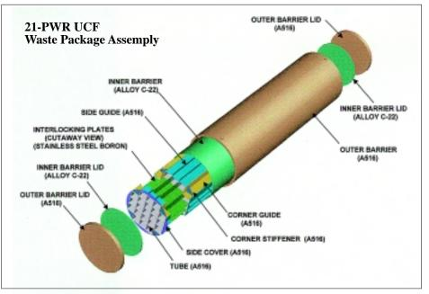
Fig. 7. The VA design for the waste package included a thick outer layer of carbon steel and a thinner inner layer of nickel-based alloy. The carbon steel provided structural strength while the Alloy 22 offered resistance to corrosion should the outer layer be penetrated.
