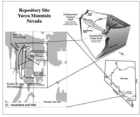
Yucca Mountain is slated by law to accommodate 70 000 MT of heavy metal although its capacity could be increased to 118 000 MT should repository requirements and legal constraints change.
