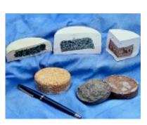
A revolutionary family of silicone-based geopolymers that can coat or encapsulate waste, facility surfaces or equipment
