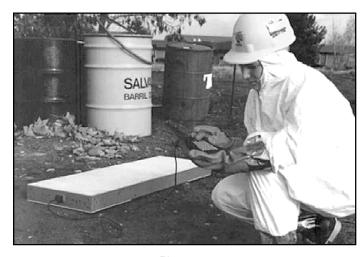
Fig. 4. The BetaScint<sup>™</sup> Fiber-Optic Sensor minimizes costly sampling and analysis by allowing a technician to locate strontium-90 and uranium-238 on soils and pavements. The conventional method obtains samples for later offsite laboratory analysis. This sensor reveals the presence of beta emitters in real time. resulting in cost and scheduling benefits. (TechID 70)
