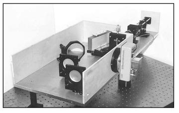
▲ Fig. 5. The Compact High Resolution Spectrometer is a versatile optical spectrometer for use in field and process applications. This real-time monitor can analyze actinides and continuously monitor EPAregulated toxic metals, uranium isotopes, and actinides in stack gases. Cost savings result from on-line process control and reducing the need for intensive front-end waste characterization. (TechID 1564)
