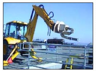
Robotics staff at PNNL constructed a wooden mockup of the Cybernetix arm to conduct cold testing and operator training.
