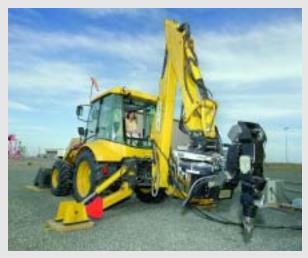
The Pit Viper integrates a typical industrial backhoe with a robotic manipulator arm controlled from a remote location, effectively removing workers from high-radiation zones within the pit area.
