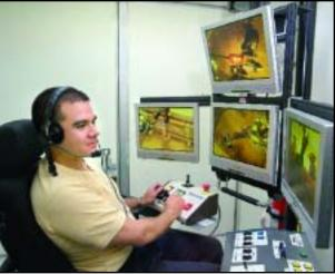
Surrounded by a bank of viewing screens, an operator uses joysticks to control dexterous movements by the Pit Viper robotic arm.
